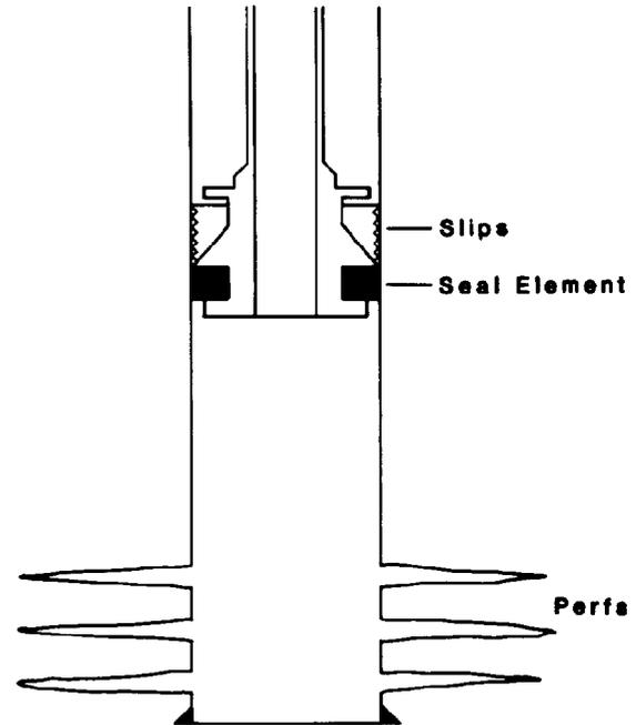
Fig. 4.2—Solid-head retrievable tension packer.
