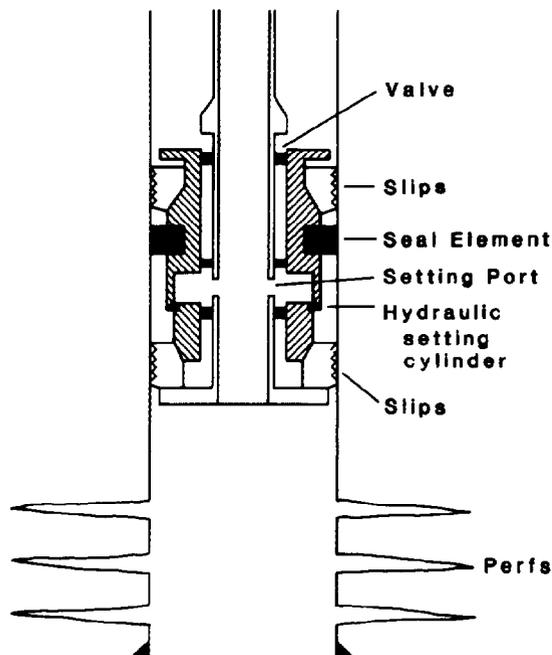
Fig. 4.7—Hydraulic packer is set by tubing pressure.
