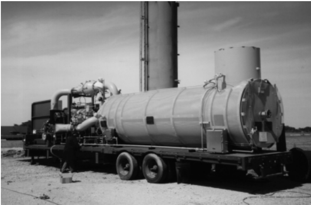
Figure 5-3—Example of Tank Mechanical Vapor-Freeing Equipment
