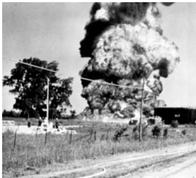
Figure G—1—Boilover of a cone-roof tank
